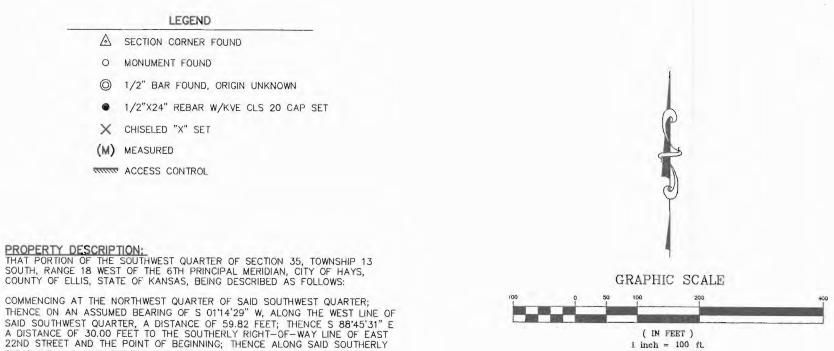
THENCE ON AN ASSUMED BEARING OF S 0114'29" W, ALONG THE WEST LINE OF SAID SOUTHWEST QUARTER, A DISTANCE OF 59.82 FEET; THENCE S 88'45'31" E A DISTANCE OF 30.00 FEET TO THE SOUTHERLY RIGHT-OF-WAY LINE OF EAST 22ND STREET AND THE POINT OF BEGINNING; THENCE ALONG SAID SOUTHERLY RIGHT-OF-WAY LINE THE FOLLOWING 7 COURSES; THENCE S 89'06'25" E A DISTANCE OF 5.00 FEET; THENCE N 46"03'55" E A DISTANCE OF 35.46 FEET;
